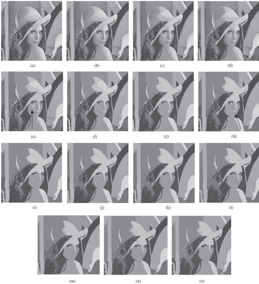
Figure 18. a) Original image (Lena), (b) Segmentation for hr = 5 and hs = 2 , 14 iterations, (c) Segmentation for hr = 7 and hs = 4 , 16 iterations, (d) Segmentation for hr = 9 and hs = 6 , 25 iterations, (e) Segmentation for hr = 11 and hs = 8 , 48 iterations, (f) Segmentation for hr = 13 and hs = 10 , 25 iterations, (g) Segmentation for hr = 15 and hs = 12 , 20 iterations, (h) Segmentation for hr = 17 and hs = 14 , 26 iterations, (i) Segmentation for hr = 19 and hs = 16 , 24 iterations, (j) Segmentation for hr = 21 and hs = 18 , 21 iterations, (k) Segmentation for hr = 23 and hs = 20 , 26 iterations, (l) Segmentation for hr = 25 and hs = 22 , 13 iterations, (m) Segmentation for hr = 27 and hs = 24 , 5 iterations, (n) Segmentation for hr = 29 and hs = 26 , 8 iterations, (o) Segmentation for hr = 31 and hs = 28 , 10 iterations. The arrows indicate the permanency of stains for those window sizes.
